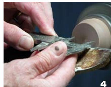
Use calipers to mark the clock diameter on the wasteblock that will become the tenon.
