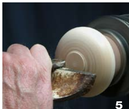
Use your spindle gouge to smooth the back of the clock body.
