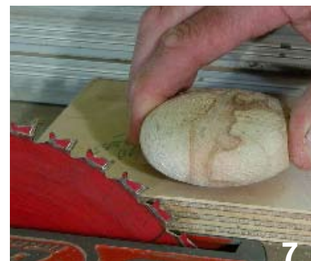
With the tablesaw blade tilted about 6 or 7 degrees, cut a flat spot on the clock body.
