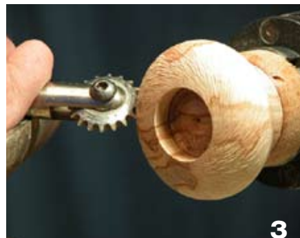
Engage the tool at the edge of the hole and move it toward the edge of the body.
