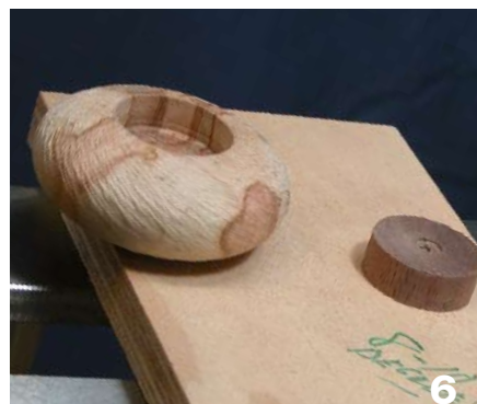
Part off a short length of the jam chuck tenon and fasten it to a piece of plywood.
