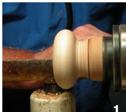
Leave a sturdy wasteblock on the back of the clock (1½" diameter shown above).
