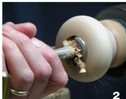
Advance the quill to bore a ¼"-deep hole to accept the clock insert.
