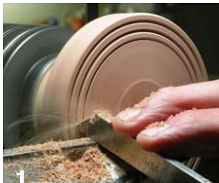
1 Use a beading tool to cut three beads into the rim of the medallion.
