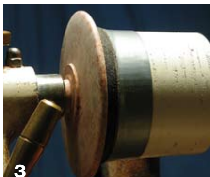
3 Insert the medallion taper into the tailstock quill and press it against the vacuum chuck.
