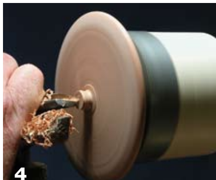
4 Back off the tailstock and carefully turn away the remaining small tenon.
