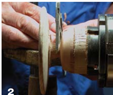
2 Turn a tapered tenon on the medallion wasteblock using calipers to check the diameter.
