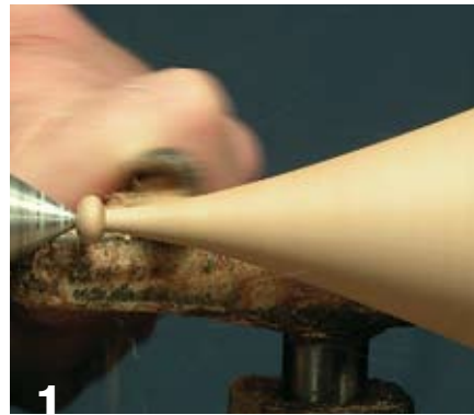
1 Use a spindle roughing gouge on its side to refine the shape of the finial.
