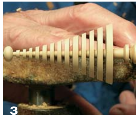
3 Create a stand for the tree and part the ornament from the chuck.
