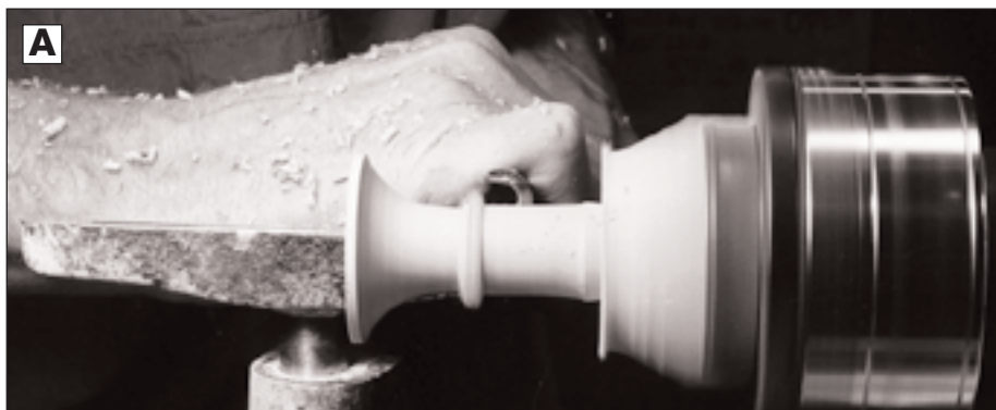
A Rough-shape the bell and refine the decorative ring around the bell.
