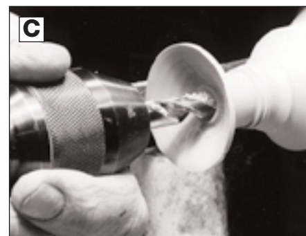
C With a 3/8" drill bit, drill the final depth of the bell.
