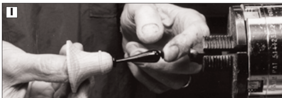
I With five-minute epoxy or cyanoacrylate (CA) glue, glue the handle into the bell.
