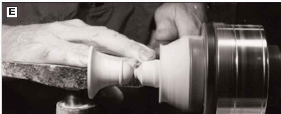
E Refine the top of the bell before parting it from the lathe.
