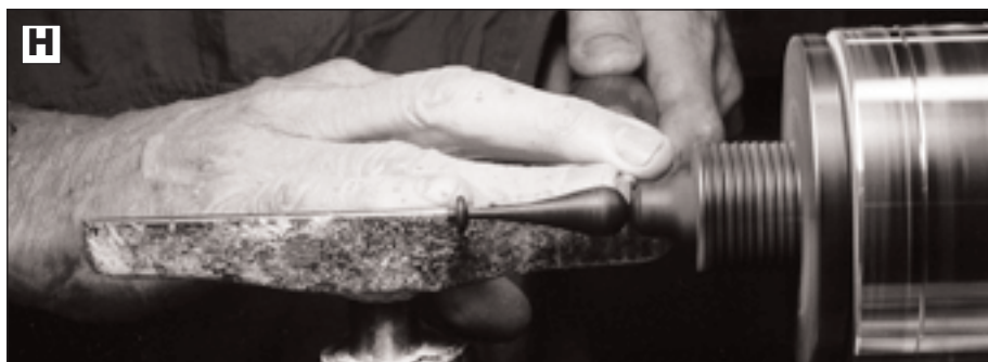
H Refine the shape of the ebony handle with a spindle or roughing gouge.
