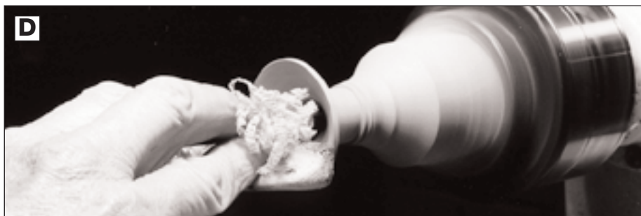
D Use a round-nosed scraper to remove the rest of the material from the interior.
