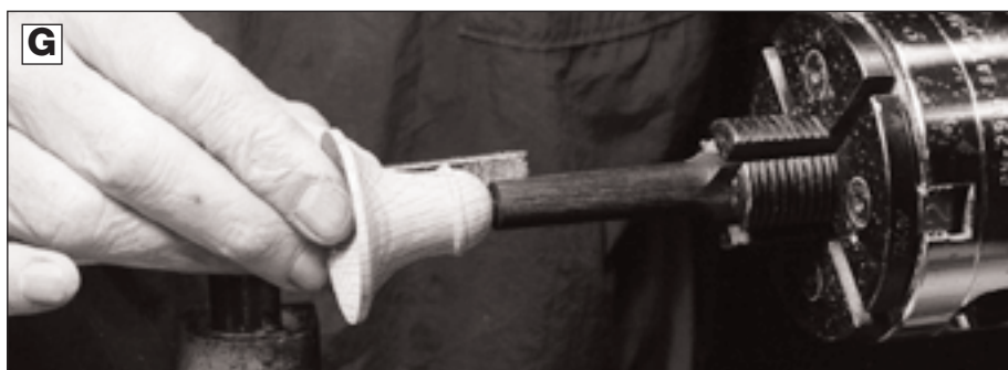
G After rough-turning the handle, check the fit of the handle tenon into the bell.
